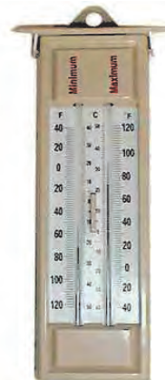
Fig 2.2 : Minimum and maximum thermometer
