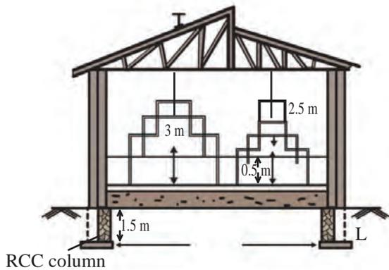
**Fig. 6.2 : Sectional view of cage system**
