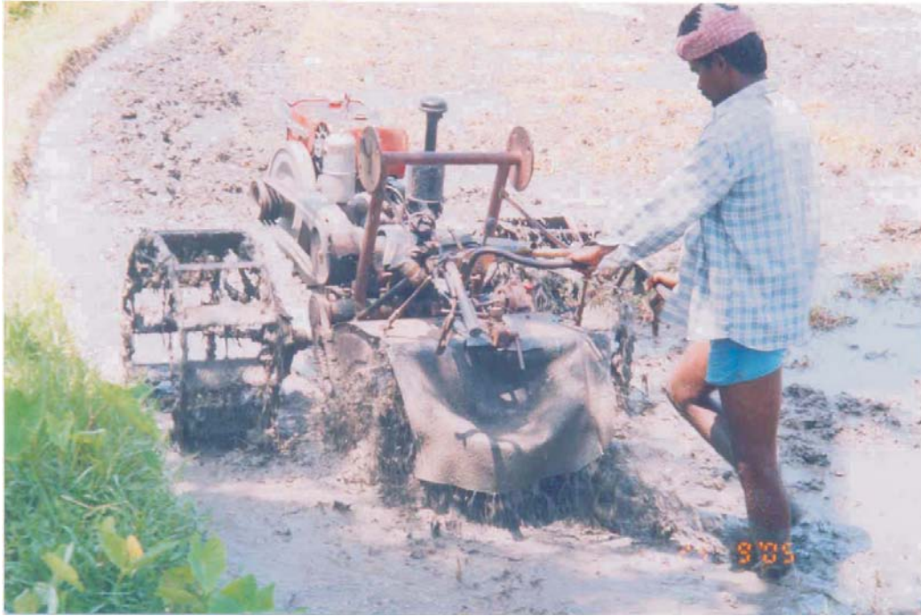
Fig. 15.1 Puddling rice field with power tiller
