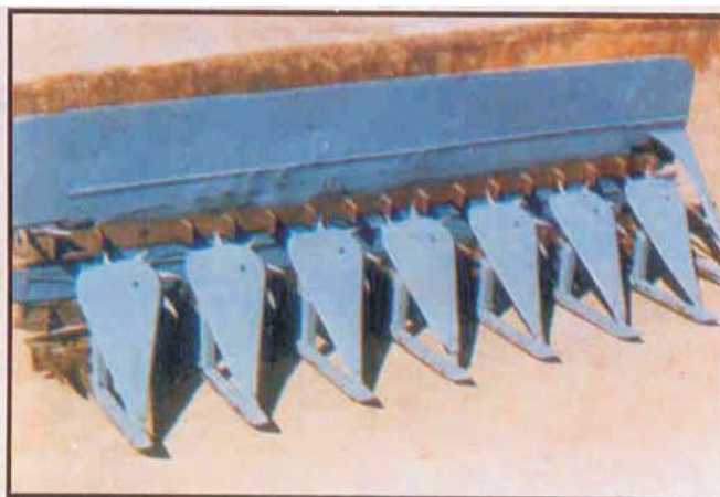
Fig. 15.11 Tractor mounted conveyor reaper
