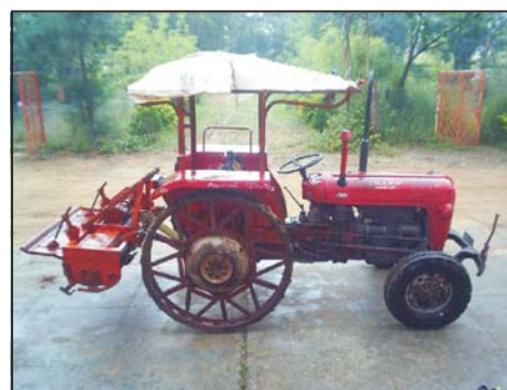
Fig. 7.2a Tractor operated rotavator
