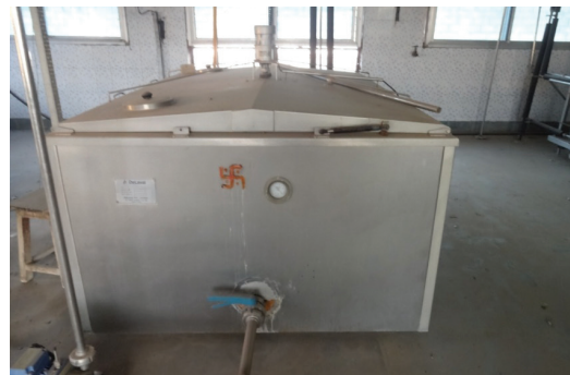
Fig. 3.5: A milk chilling tank of 1000 litre capacity
