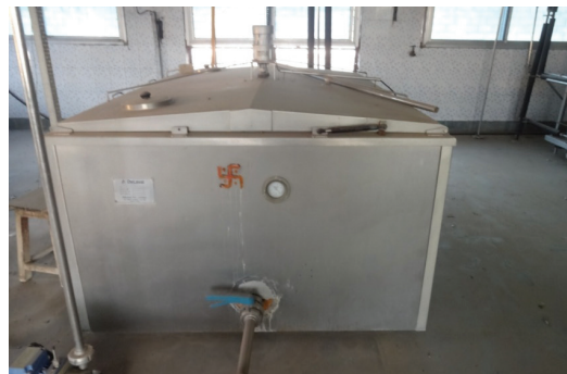
Fig. 3.5: A milk chilling tank of 1000 litre capacity
