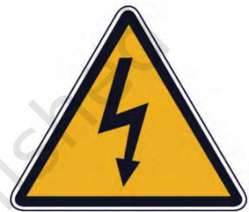
Fig. 7.6: Electricity hazard sign
