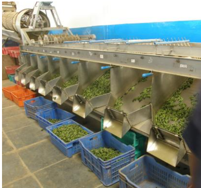
Fig. Grading of Gherkin through divergent rope after deflowering
