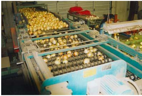
Fig.:9 Sizing by rollers of increasing distance between them.
