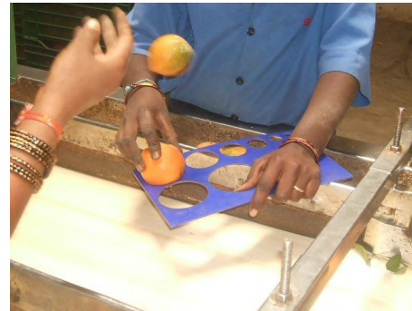
Fig.:11 Sizing with rings of known diameters
