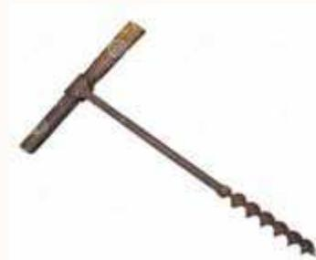
**Fig2. Screw auger**
