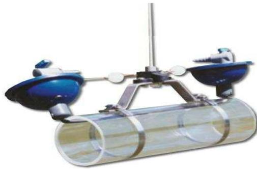
Fig.1. (a) Vandorn sampler
