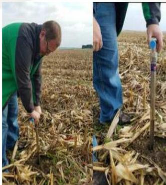
**Fig 3. Collection of soil sample using soil probe**
