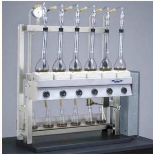
**Fig. 9 Kjeldahl Digestion Assembly**
