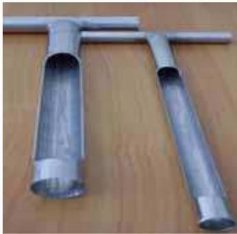
**Fig 1. Tube auger**
