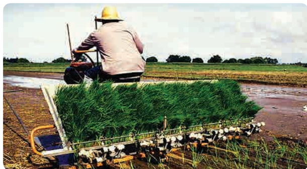
Fig. 1.11 A) Mechanical paddy transplanting
