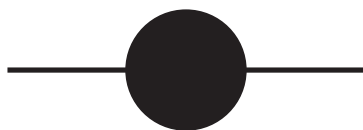
Fig. 1.34: Symbol for sprinkler – full
