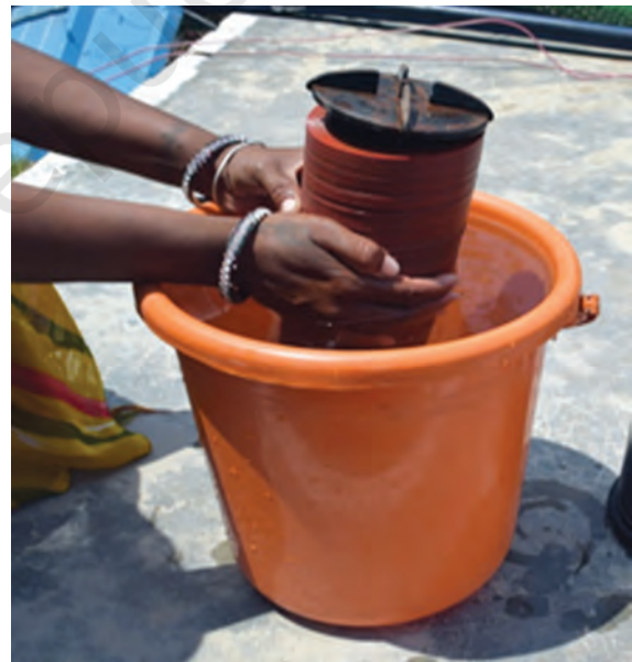
Fig. 3.8: Cleaning of disc filter
