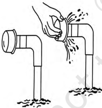
Fig. 3.5: Main or sub-main flushing
