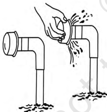
Fig. 3.5: Main or sub-main flushing
