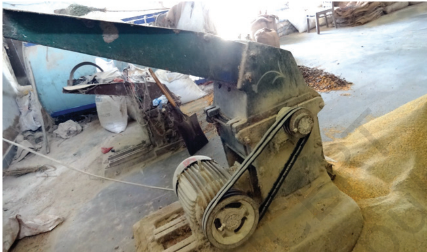
Fig. 4.9: Electrical feed grinder
