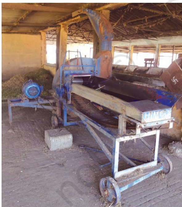
Fig. 4.8: Electrically operated chaff cutter
