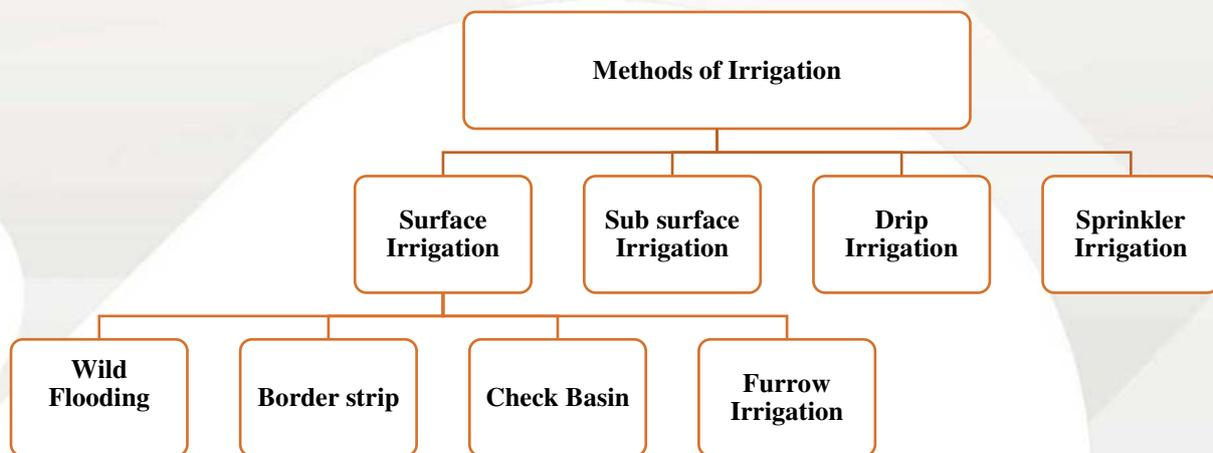
**Fig 1 Classification of different method of irrigation**
